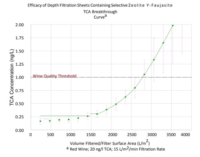
The breakthrough curve shown was generated using a number of commercial pads produced on various production dates.
