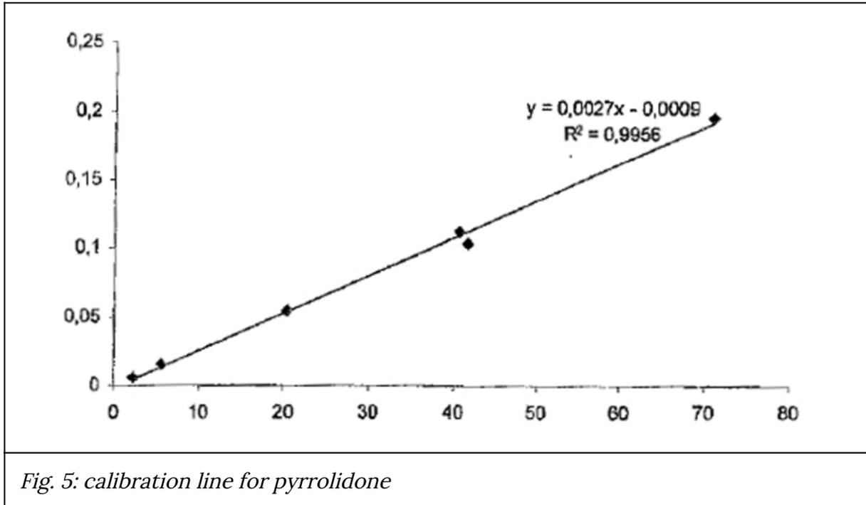
*Fig. 5: calibration line for pyrrolidone*
