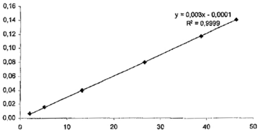
*Fig. 4: calibration line for vinylpyrrolidone*
