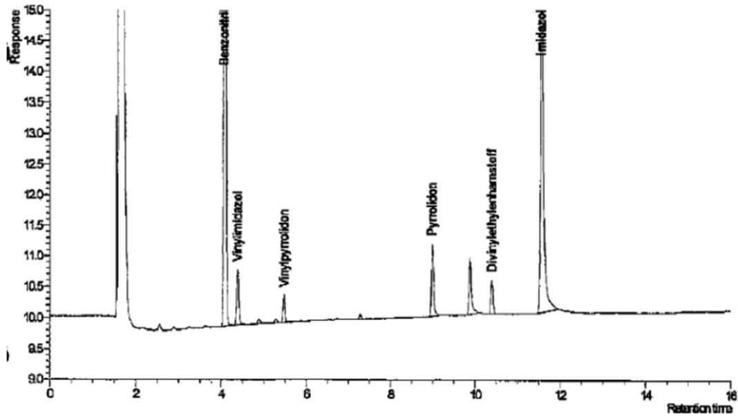
*Fig. 2 Chromatogram of the copolymer extract (with internal standard), supplemented by 2.1 µg/g of vinylimidazole, 2.1 µg/g of vinylpyrrolidone, 3.9 µg/g of pyrrolidone, 2.1 µg/g of divinylethyleneurea, and 12.7 µg/g of imidazole.*
